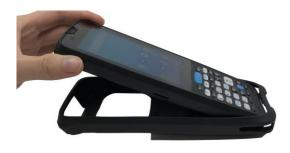
2). Make sure HT330 is secured in the boot case.
