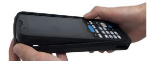
2). Pry the boot case from the other edge of top corner, and pull HT330 out.
